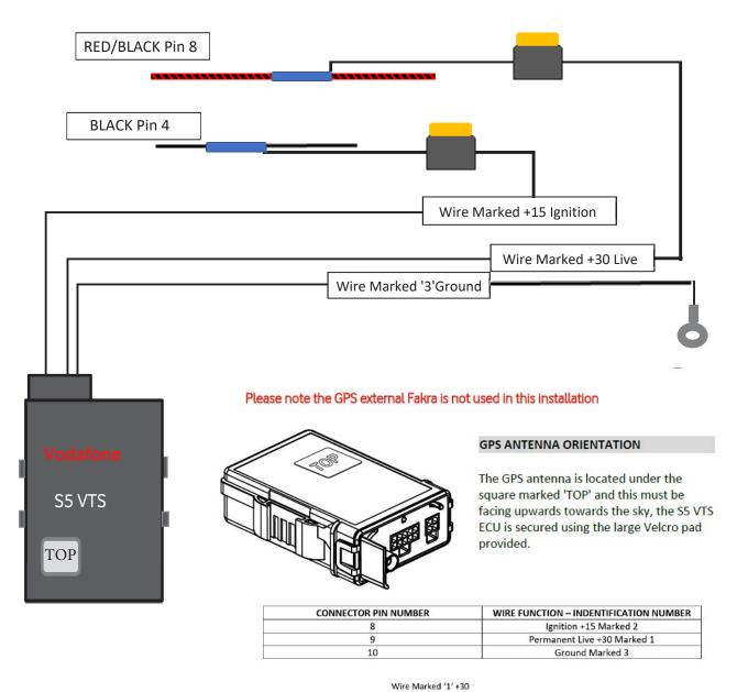
**PLEASE NOTE:** the two wires marked 'ECI' are not used for this installation and must be cut and insulated.
