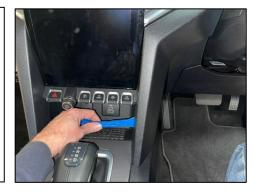
Apply some masking tape to the surface of the trim panel where the switch will be installed, then measure 80mm from the corner of the trim and draw a line at a 90-degree angle. (See Image A)
