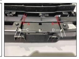
14a.) Once you have established the correct bracket orientation, rest the mounting brackets in position over the back of the grill.
