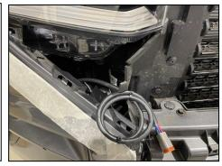
Connect the two driving light connectors to the wiring harness then carefully feed any excess cable into the space below each headlight.
