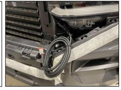
Route the other driving light cable up the inside of the Left-hand headlight, following the vehicles existing wiring harness and secure with a cable tie. (See Image>)
